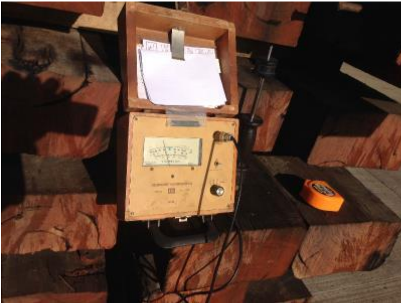
Moisture Metre being used on 300x150 hardwood Image used with permission
