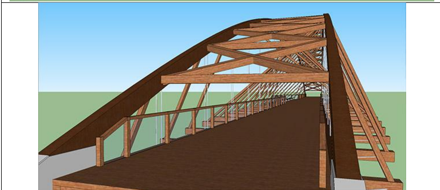
120m Clear Span Timber Bridge
