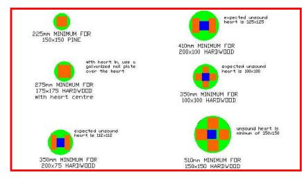
The inner heartwood (wood within 50 mm of the pith)of Australian hardwoods is usually less durable and softer the than outer Under AS heartwood. 2082 heart is only permitted in structural timber when the size is least 175x175mm. at (Designers should be
