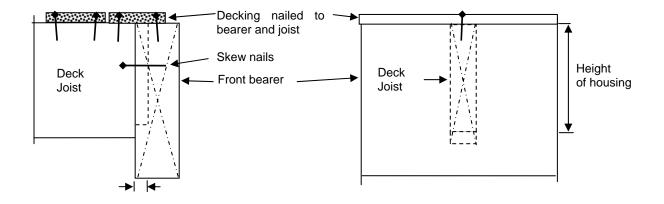
All Timber Queensland Members should note this potential failure issue with the construction method used and should include it with all the other issues (hand rail sizes and fixings, timber decay etc) in respect to any inspections undertaken on decks in the future.
