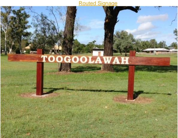
Infrastrucxion has competitive pricing on hardwood routed and painted signs. This example is is made from 300x50 dressed spotted gum. The top of the sign is rounded to shed water as in our handrail profiles. The sign is mounted onto Pioneer Posts, The stainless steel caps are not fitted yet. Contact us about your signage and post requirements.
