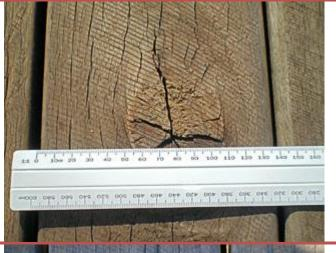
**Sound Knot**, At least it was when it was cut and that is how you have to imagine it when you grade it, not as you see it now, It measures about 60mm across a face of 145 when laid, i.e. 40% of the face. The allowance for knots in AS2082 in unseasoned timber for the different stress grades is
