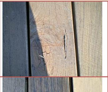
Combination Defect. When grading these defects the width of the knot is added to the width of the shake. This combination defect is over 50% of the piece
